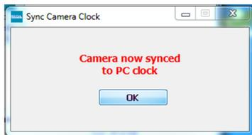
**NOTE:** You will need to sync the camera module again when seasonal time changes occur. The camera module will not automatically adjust the time. Syncing the camera module to a Windows computer ensures you have the proper time.
