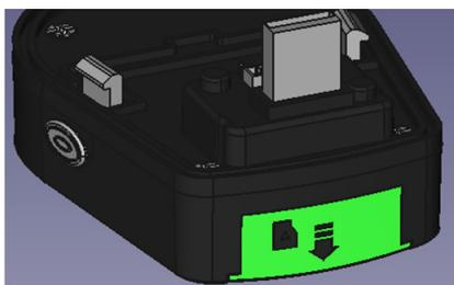
2. Locate the sliding cover on the back of the camera module with a picture of a micro-SD card.
