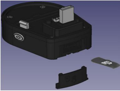
5. Grab the back end of the micro-SD card with your fingertips and remove it from the camera module. To replace the micro-SD card, push it back into the slot on the back of the camera module. Be sure it is in the correct orientation! This can be seen in the image below.
