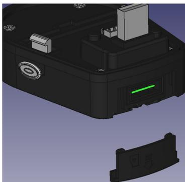
3. Use a Phillips-head screwdriver to remove the screw in the bottom of the cover, then slide the cover off the camera module. You will see the back of the micro-SD card.
