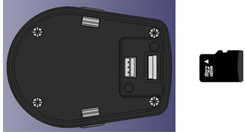
**NOTE:** The back of the micro-SD card should not be flush with the gasket. It should be slightly deeper into the camera module so it is almost hard to touch with your finger. If it looks flush with the gasket after hearing it click, take it out and try again. It may not record properly if it is not inserted correctly.
