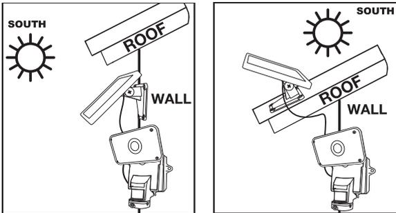
The solar panel will charge the battery pack on cloudy days; however, the total battery charge will be less than it would be on a sunny day. Placing the solar panel in a shaded location or behind a window will prevent the battery pack from charging and the video camera floodlight from operating.
