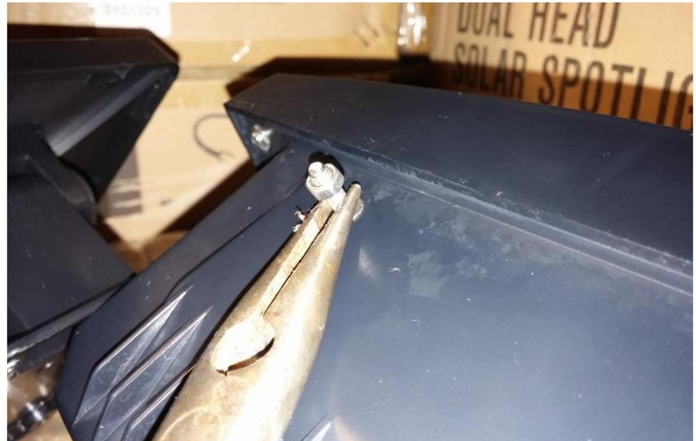
While still holding the bolt with the needle-nose pliers, place one hole of the solar panel over the bolt. The small size of the needle-nose pliers should allow clearance to do this. Continue to maintain your grip on the bolt with the needle-nose pliers.
