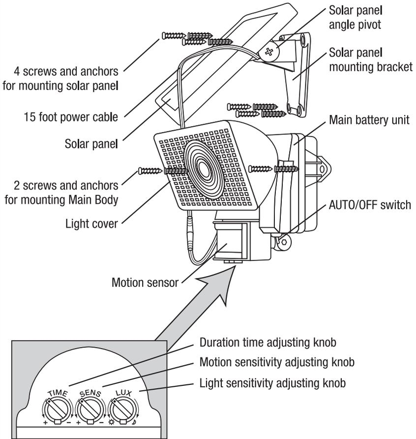
Once you have identified all parts, connect the solar panel to your Solar Security Light by plugging the 15 foot cord into the cord attached to the front of the Solar Security Light. Turn and twist the cords while pressing firmly together until they are attached tightly.
