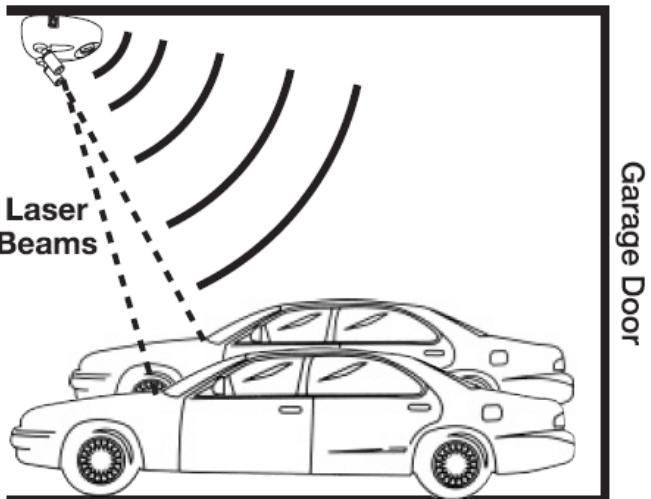
6. When either of your cars first enters the garage, the motion detector will turn on both lasers. Drive forward until the laser beam for your vehicle hits your pre-determined spot indicating that you are parked in the correct position. Both lasers will turn off automatically after you are parked.
