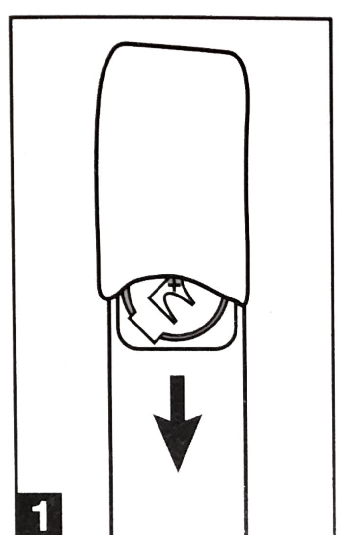
Gently pull battery holder out from beneath the elastic pouch on back.
