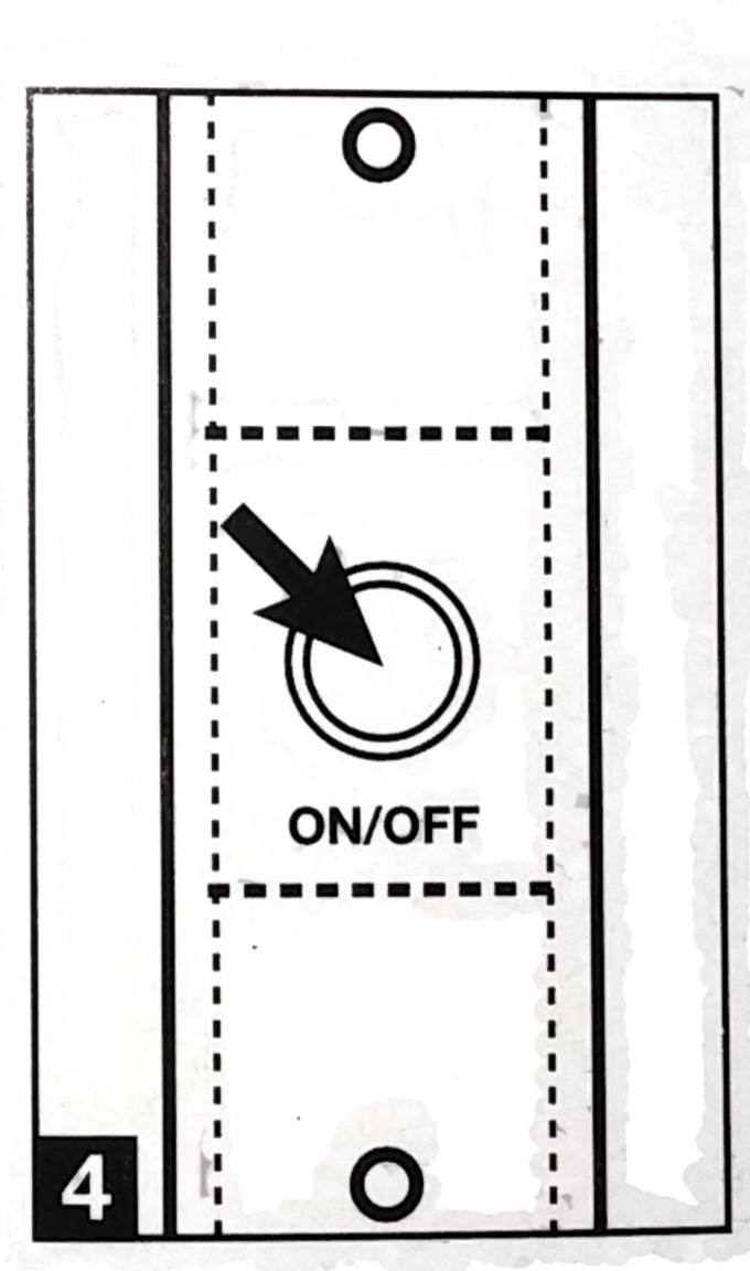
Turn safety band over and press ON/OFF button to turn on flashing lights.
