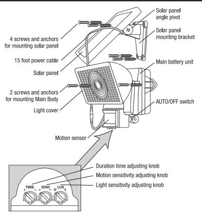
Once you have identified all parts, connect the solar panel to your Solar Security Light by plugging the 15 foot cord into the cord attached to the front of the Solar Security Light. Turn and twist the cords while pressing firmly together until they are attached tightly.
