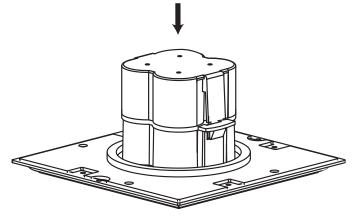
6. Reassemble the *LED Outdoor Wall Sconce* by replacing the top cover and re-installing the two thumb screws. Tighten the thumb screws by hand as tightly as possible to ensure a waterproof seal.
