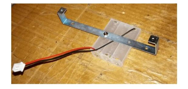
Insert 3 rechargeable AA batteries into the battery tray.
