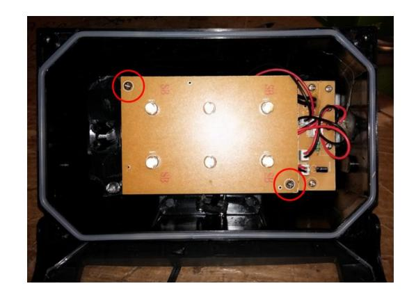
Pull the LED board out. Be careful not to sever the wires connecting the LED board to the control board still within the body.
