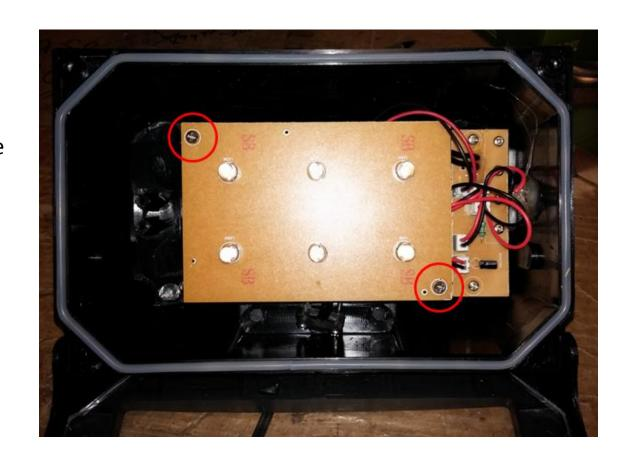
Place the reflective plate back over the LED board. Rotate the face of the light upwards so it closes. Insert and tighten the screws on the front. Then tighten the screws on the sides of the faceplate.
