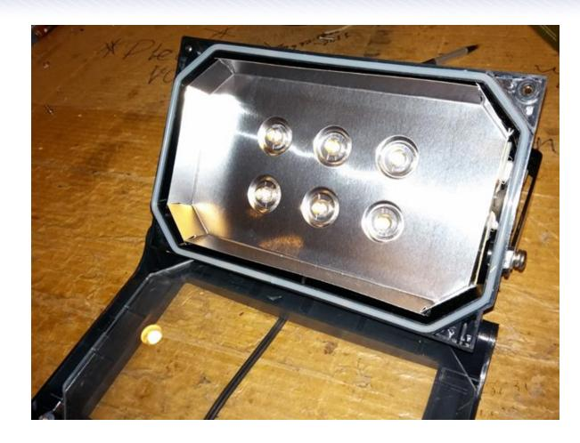
Pull the reflective plate out of the light. It should lift right out and expose the LED board. You will see two screws holding the LED board in place (circled in red). Remove them.
