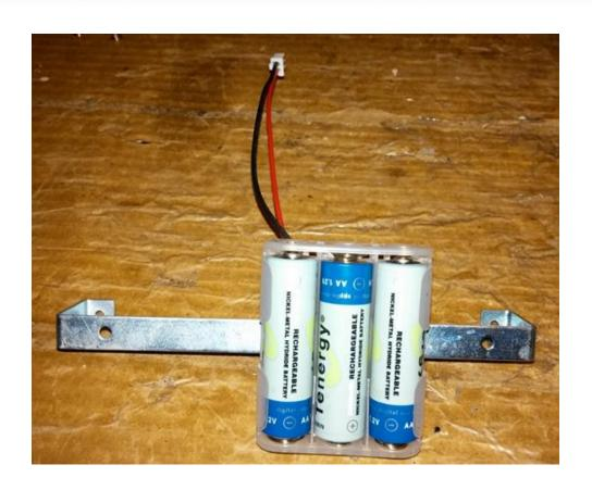
Place the bracket back into the body of the light. Be sure the plug from the battery tray is on the same side as the control circuit board.
