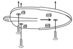
**CAUTION: DO NOT USE DOUBLE-STICK TAPE TO MOUNT THE UNIT TO THE CEILING. MOUNT SECURELY WITH SCREWS ONLY.**
